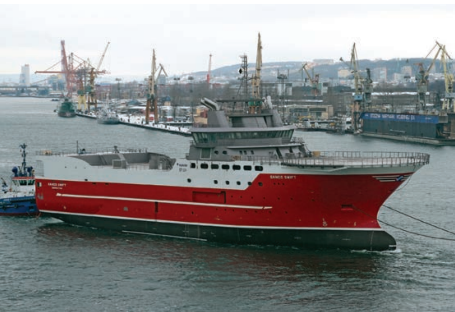
Partially outfitted hull, built at Crist yard, of Sanco Swift - seismic survey vessel completed at Kleven's Myklebust Verft AS.
