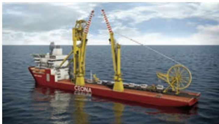
The ship will be required to lay fixed and flexible pipes on the seabed in water as deep as 3000 metres.
