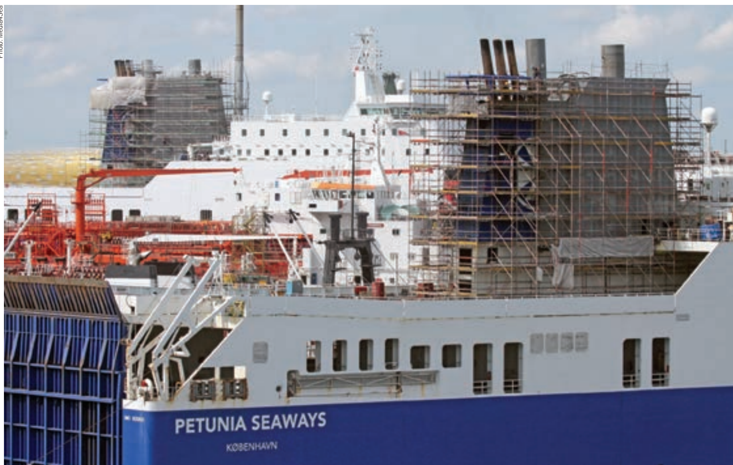
Petunia Seaways during scrubbers installation. In the background another DFDS Seaways ship while the similar operation was being performed.
