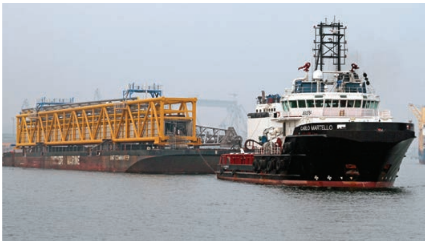
Transport bridge and flare tower from Vistal for Eldfisk platforms complex expansion project.
