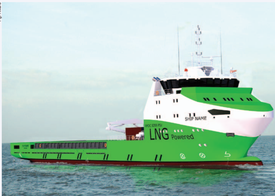
Platform Supply Vessel of the RMDC LNG DF 8286 design.
