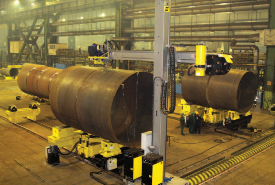
The first modern production line for the wind towers made in Gdansk, opened late 2010, was arranged in the part of the largest production hall in Middle-Eastern Europe (65 000 sq m under one roof) formerly utilized mainly for shipbuilding production.
