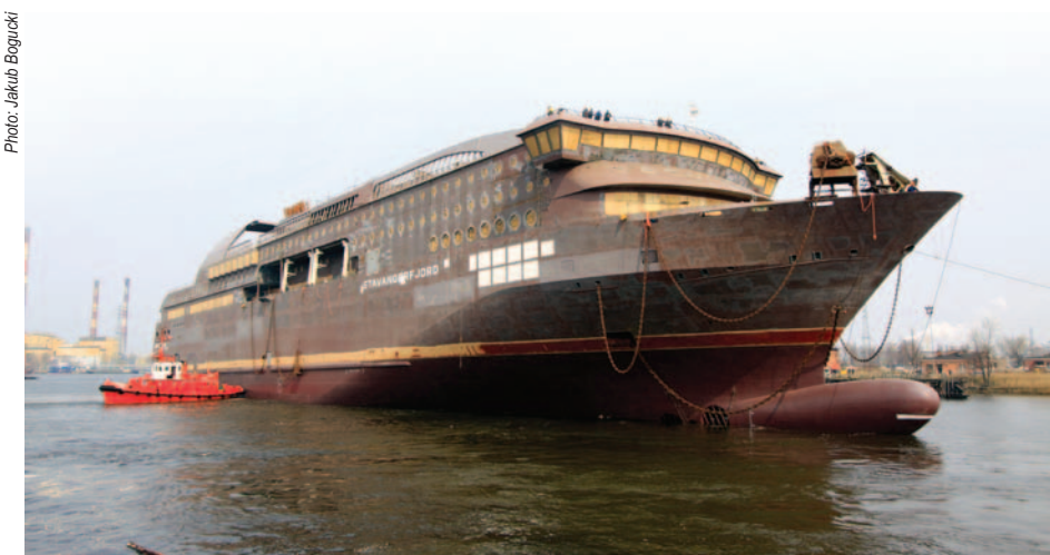
Partly equipped hull of Stavangerfjord launched at Gdansk.
