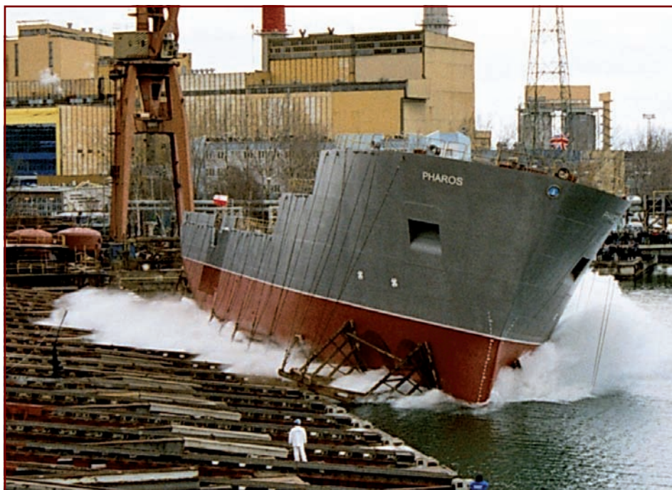
NLV Pharos was side-launched at Northern Shipyard in February 2006.
