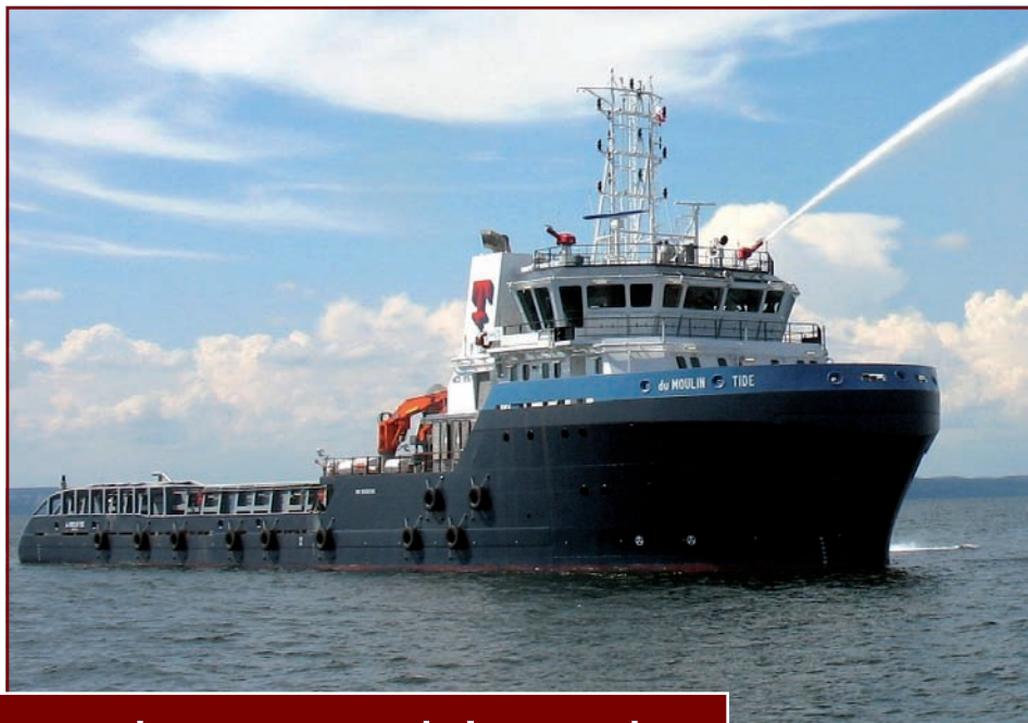
The 120 T bollard pull AHTS ship de Moulin Tide , during sea trials.
