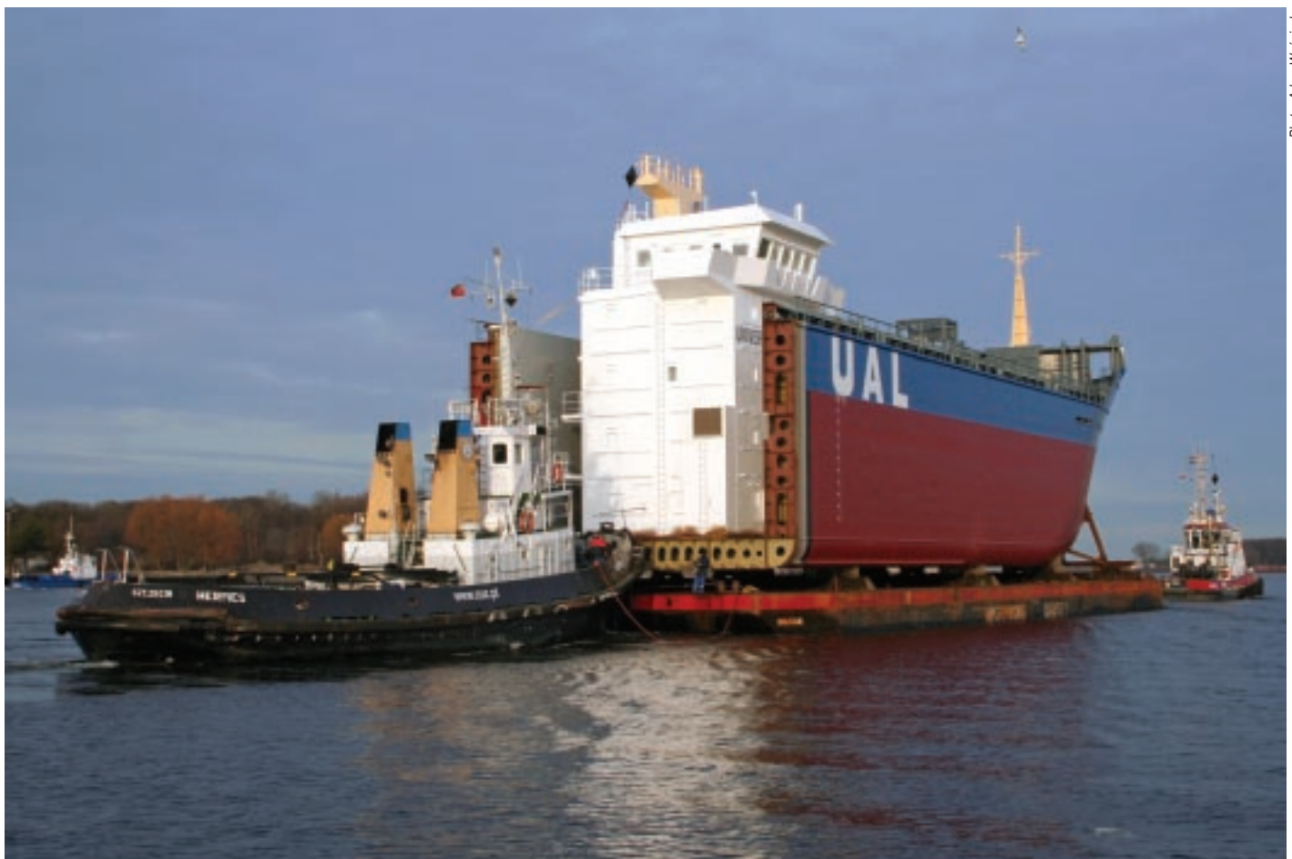
Bow part (roughly half of the length of a hull) of partly outfitted hull of a multipurpose cargo ship „carrying” its own superstructure in its hold. This is a shipment from Szczecin based Partner shipyard for a Dutch shipyard and the ship itself is a 119 m long and 7755 tons deadweight UAL Cyprus.
