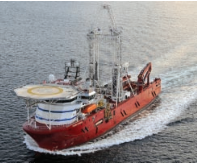
Fugro Synergy, of which the partly outfitted hull was supplied by Gdansk Shipyard, was awarded, in 2010, the title of the „Ship of the Year” from „Offshore Support Journal”. Fugro Synergy, features 4400 deadweight tonnage and is 104 m long. It is advanced, complex geotechnical drilling and well workover vessel.
