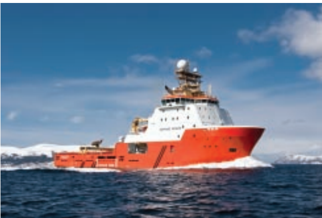
Normand Ranger is a powerful AHTS of 2010, with partly outfitted hull supplied by Crist Shipyard. The ship's deadweight is some 4500 t and length - 91 m.
