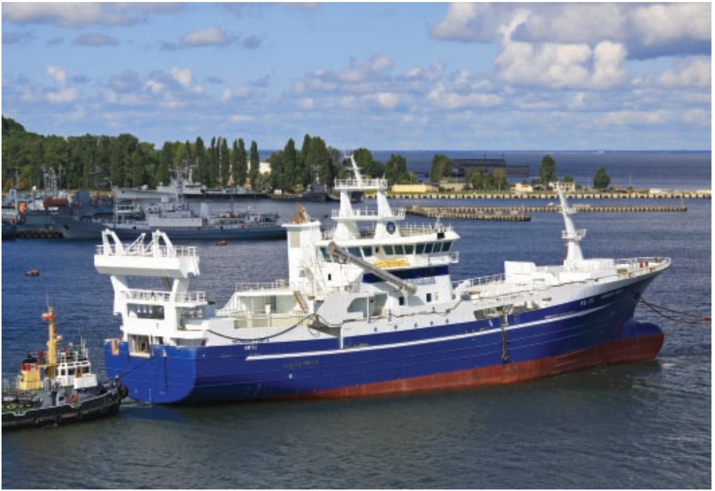
Partly outfitted hull of the 82 m long multipurpose fishing vessel (seiner and trawler) Trondur i Gotu of 2010, featuring 3500 t deadweight, has been delivered by Naval Shipyard Gdynia to Danish yard Karstensens Skibsværft of Skagen and ultimately destined for Faroese owner.
