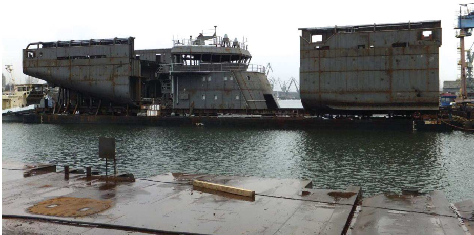
Operation of loading of hull blocks for Simek yard newbuilding no. 126 onto Simek II heavy-lift pontoon-barge at Maritim Shipyard in Gdansk.
