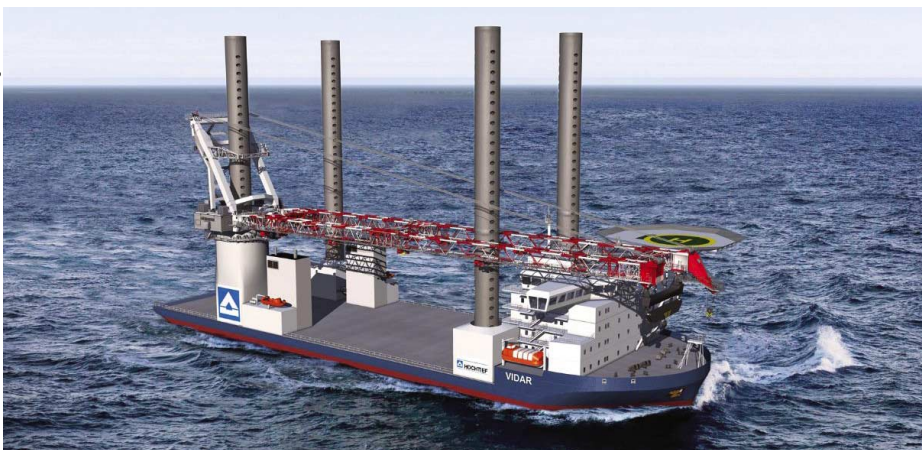
Computer graphics rendering of the new special-purpose jack-up vessel Vidar.
